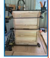
worry about it at this stage. At this stage you also need to install the 22mm fillers and entrances. These can simply be glued in as they will be 'wedged' between the two front covers.
