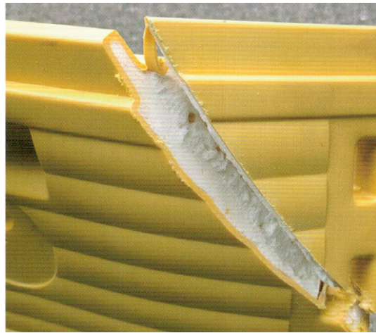
Doubled walled structure with insulation and latch handles
